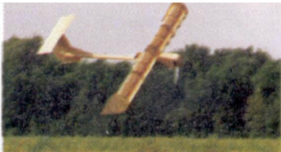
**A FanWing model in flight**
